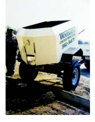
We have both 1 yard and 2 yard Carts Tilt-up container for easier dumping 1 Yard Cart has surge brakes 2 Yard Cart uses electric brakes 2-5/16" ball or pintle hitch 4,000 psi concrete mix for all carts Concrete Volume Formula (input all numbers in inches) Cubic Yards = Length x Width x Height / 46,656
